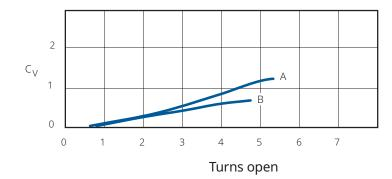
A =  $\frac{1}{4}$  inch (6.4 mm) orifice, valve  $C_V$  1.4 maximum B =  $\frac{3}{16}$  inch (4.8 mm) orifice, valve  $C_V$  .83 maximum
